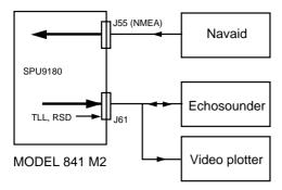
The position data from navaid can be used for the echosounder if a video plotter is not connected.
